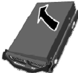
9. Fold up the flap near the back of the hard-drive tray.
