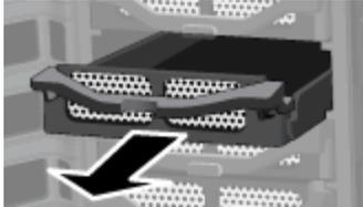
7. Flex the back of the right side-rail and withdraw the back pin from the hard drive by gently pulling the side-rail down and away.
